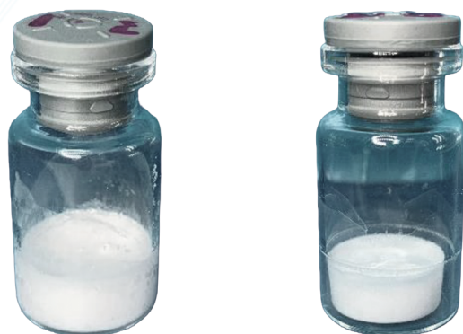
Figure 1 Lyophilised Cakes. Left Mannitol - Right Dextran
