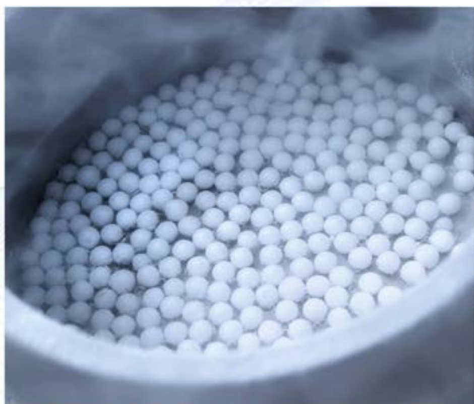
Figure 2 : With dual nozzle option up to 7,000 beads can be generated per hour
