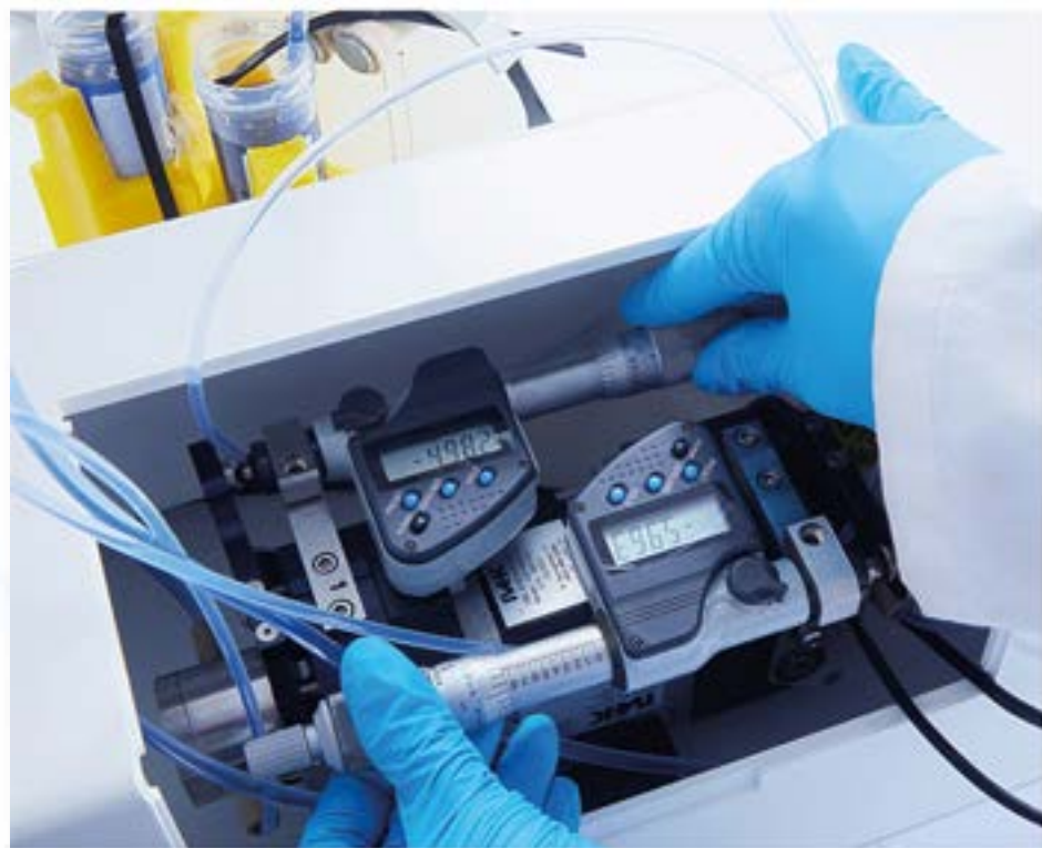
Figure 1 : Built in pump and adjustment controls. Volume precision 0.10%
