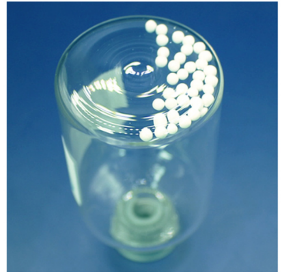
Figure 1 Lyobeads held at the bottom of the vial. The electrostatic charge generated by using glass vials is strong enough to prevent gravity from dislodging the lyobeads
